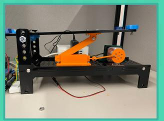
The components of the mechanism were all designed within AutoDesk Inventor, then placed into an assembly that included a model of the hopper that would be used. All components were then 3D Printed an assembled into its final design.
